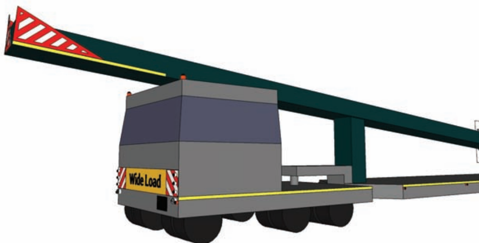
Requirements for end and side projection markers for a forward and rearward projecting load
