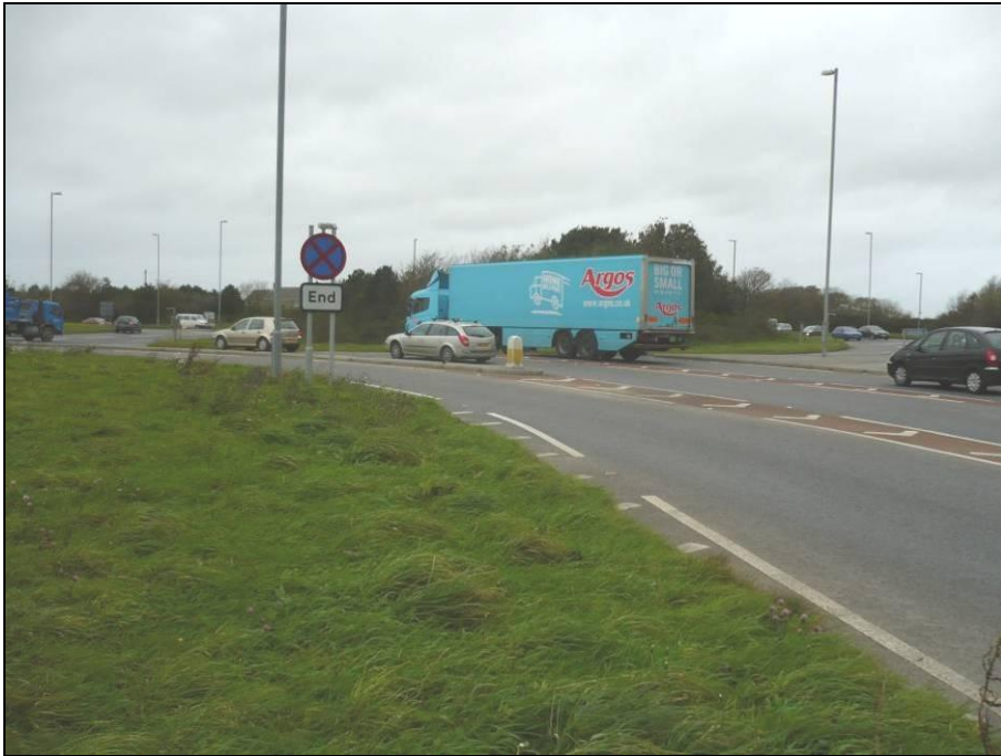
Figure 2.3 – Segregated left turn lane on the A390 approach with merge onto the A30 southbound.
