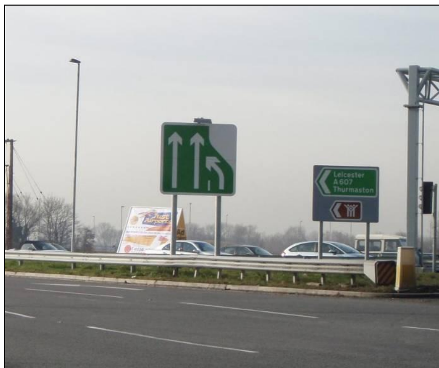
Figure 2.4 – Illuminated Merge Sign
