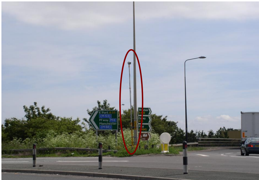
Figure A1 – Turning Count Survey using Telescopic Mounted Video Camera
